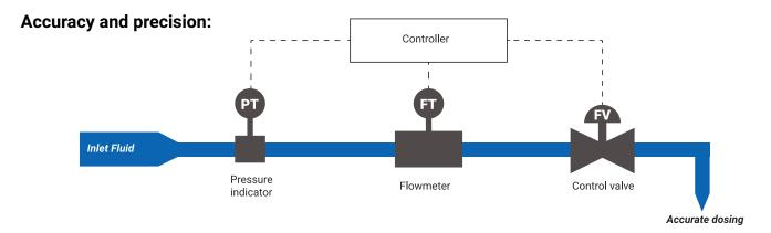
**Precision and accuracy of flow control can only be achieved with a control loop.** This control loop is programmed integrating inputs and outputs of the flow control equipment.
