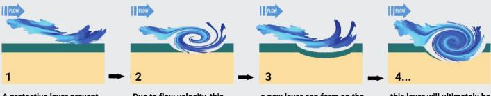
A protective layer prevent stainless steel from corroding
