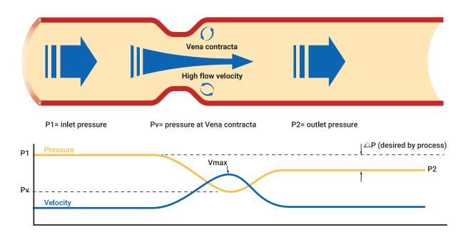
In a control valve, the flow is forced through the control valve orifice by the pressure difference across the valve. The actual flow area is smallest at the point called the vena contracta.
